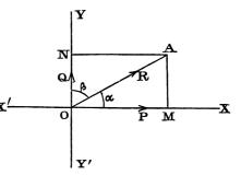
\*22. (Fig. Art. 21.) To find the resultant R in terms of the components P and Q, and to find P and Q in terms of R.
